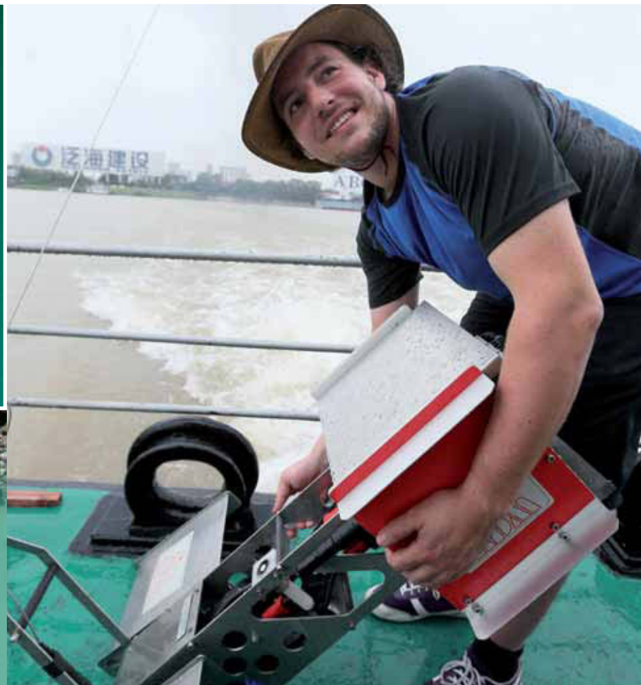
Andreas Holbach (photo on the right) of the Institute of Mineralogy and Geochemistry (IMG) holding the MINIBAT developed for pollutant analysis in the Jangtse river. It is dragged by a ship and executes the measurement at the depth desired (see above)
