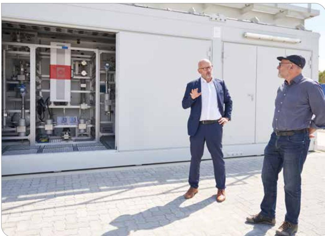
age system, forming an autonomous PtL plant. At a depth of about 40 meters in the open sea, the containers will then start offshore operation as part of the H<sub>2</sub>Mare hydrogen lead project funded by the Federal Ministry of Education and Research (BMBF).
