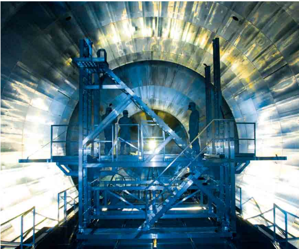
View into the main spectrometer of KATRIN: For the installation of the wire electrode system, the steel tank was made accessible for persons and equipped with a mobile scaffold
