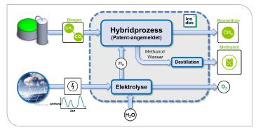
Fig. 2: Illustration of the hybrid process: In the example shown, the CO2 contained in the biogas is separated, upgraded to biomethane, and then used for methanol synthesis.
