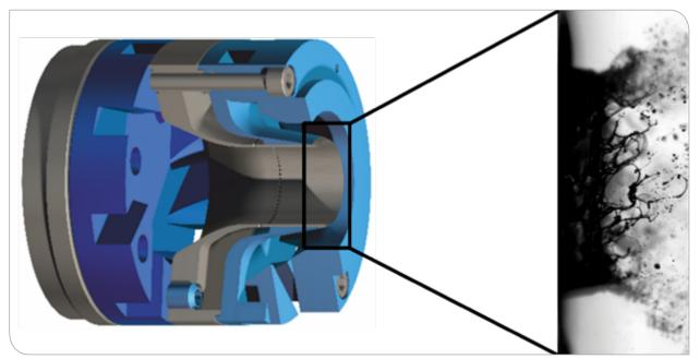
Typical injection nozzle and photography of the atomization process
