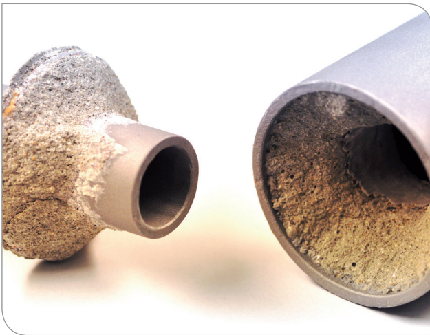
Fraction surfaces of two hollow sections (35 mm and 76 mm in diameter) joined by means of the new hybrid bonding technology (bonding gap thickness 17 mm / overlapping length 45 mm). This connection meets highest load capacity requirements (static load capacity 110 kN) and can also compensate larger tolerances
