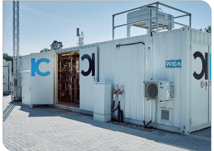
Container for the production of e-fuels. (Photo: Cynthia Ruf, KIT)
