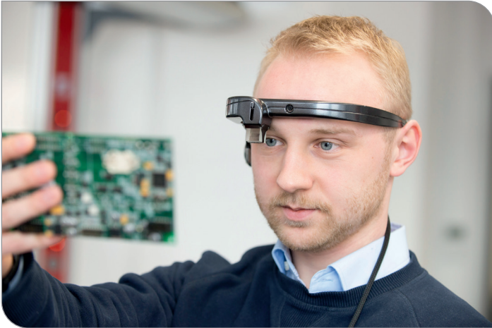
Augmented-reality glasses allow the digital assistant to understand what the user sees. This allows humans and machines to communicate in real time (Photo: Tanja Meißner/KIT).
