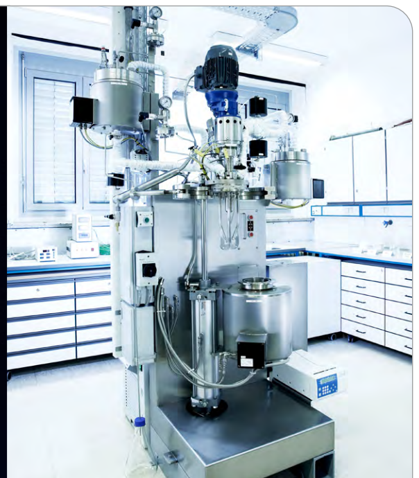
Left: View into the lab-scale rotary kiln. The fine concrete fraction and limestone react to belite cement clinker in 90 percent CO 2 . Right: Lab autoclave for fixing CO 2 in coarse crushed concrete.
