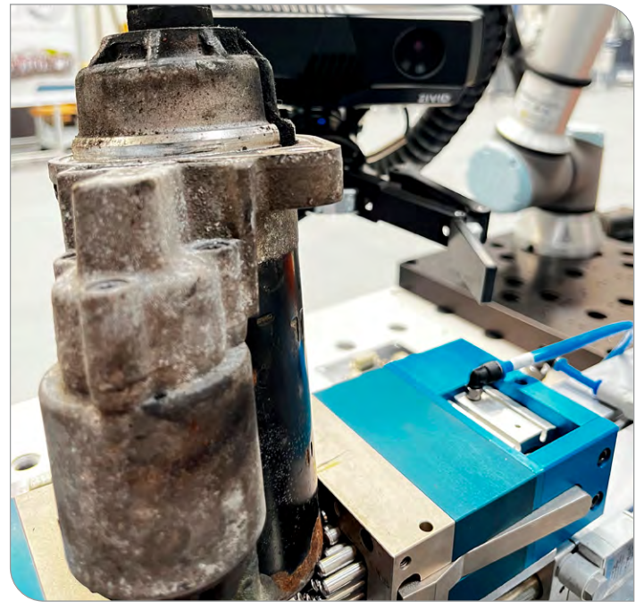
Inspection station with robot arm and rotary table.
