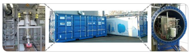
Prototype consisting of the methanation module (container on the left) and the electrolysis module (container on the right)
