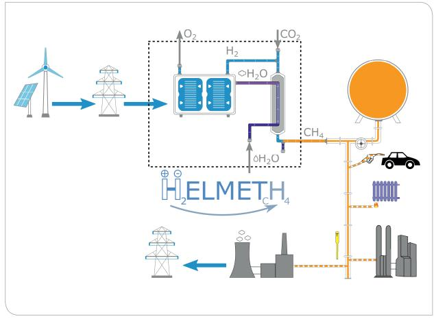
Schematic HELMETH Power-to-SNG Process
