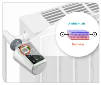
Thermoelectric generators for the autonomous supply of measurement electronics, such as a smart radiator thermostat
